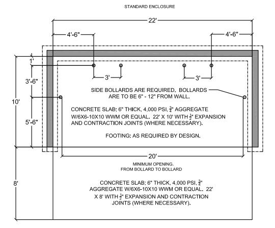
APRON REQUIRED IN FRONT OF EACH ENCLOSURE 6" WITH REINFORCING TO WITHSTAND 57,000 LBS.
