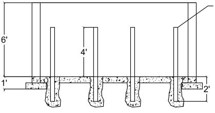
APRON REQUIRED IN FRONT OF EACH ENCLOSURE 6" WITH REINFORCING TO WITHSTAND 57,000 LBS.
